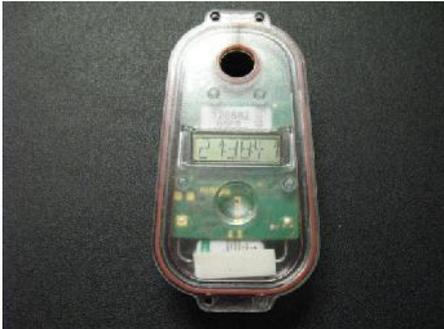
Wake up one of the existing controls with an SI card and check the time on the readout underneath the control. Compare this to the time on the PC by clicking on the clock in the lower right hand corner so that seconds can be viewed.
