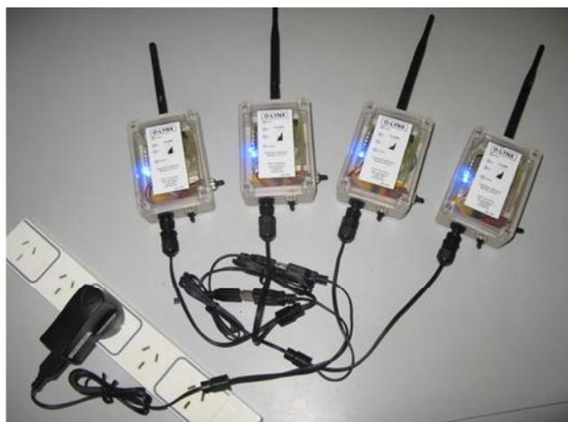
O-Lynx radios with higher capacity batteries have also been used on adventure races. These provide the ability to run continuously for at least 48 hours.
